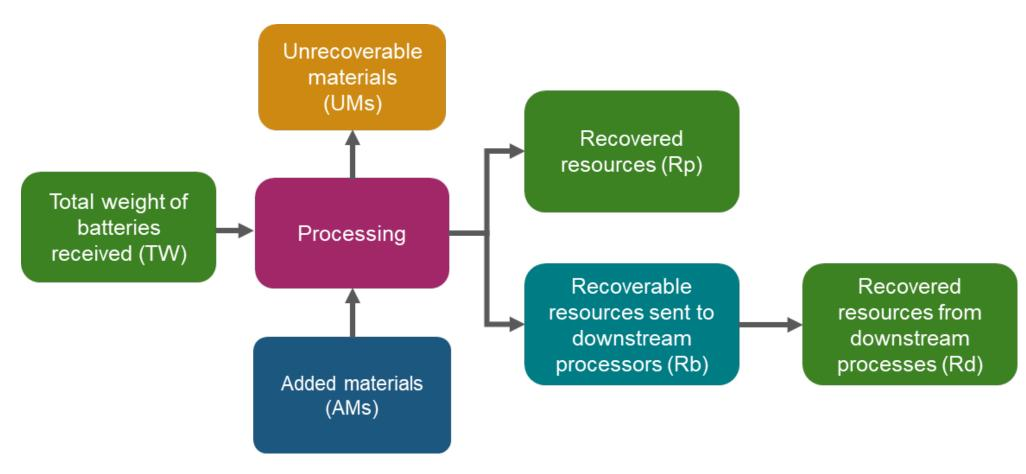
**AMs** are materials used in the process and incorporated into the outbound resources. The weight of these material must also be accounted for in the outbound materials.
