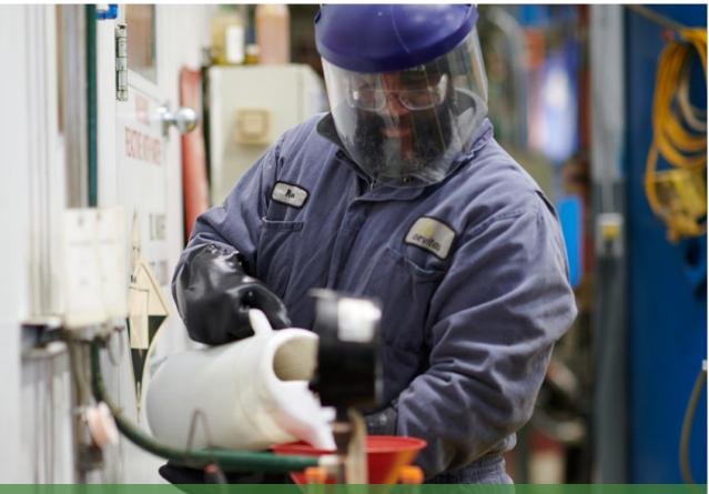
Ryan Bonner conducts tests on recovered transformer oil at a transformer oil recycling facility.
